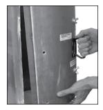
4. Insert the door into the opening at an angle and then center the door.
