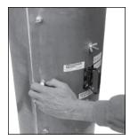
5. Tighten center wingnuts and bolts with washers.
